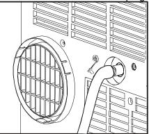
2. Connect a drain hose to the upper drain port. (Some models may have a threaded valve for a garden hose. You may need to purchase an adapter.) The portable air conditioner will now drain through the drain hose. Please note that this unit has no drain pump; all water will drain with gravity only, i.e., only "downhill."
